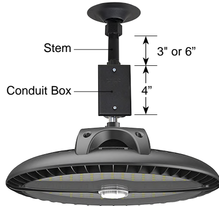
Pendant Mount 3" or 6" Stem Includes 4" Conduit Box and Swivel Canopy
