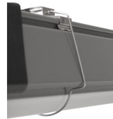
Safety Bail (SFB) Bail Snaps around the fixture into the Mounting Bracket for Additional Security/Support (316 Stainless Steel) *Sold by Each / *Required for NSF Rating
